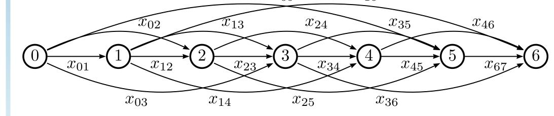
One-dimensional packing problems can be solved as a minimum flow between vertex 0 and vertex W with demand constraints.
